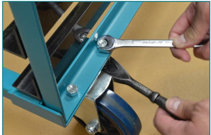
Figure 8. Attaching non-locking rear casters to bottom cross members and upright.
